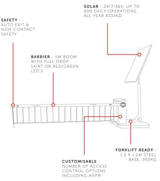
For use when only vehicle access needs to be controlled. The 5m barrier can be put into place on a forklift and be working immediately, meaning once on site, security can resume or start asap.
