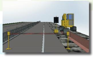
Two sensors are located at the beginning of the acceleration zone within the works area, with an HD Compact VMS deployed after the sensors which informs the works driver to wait there. Once the sensors are triggered by the works vehicle the message on the HD Compact changes to tell the driver to "Merge when safe"
